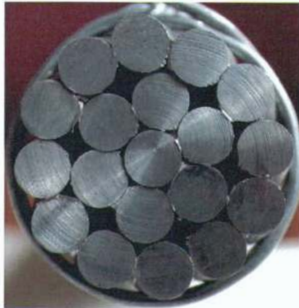
Photo 1 Cross-sectional view of the tested conductor
