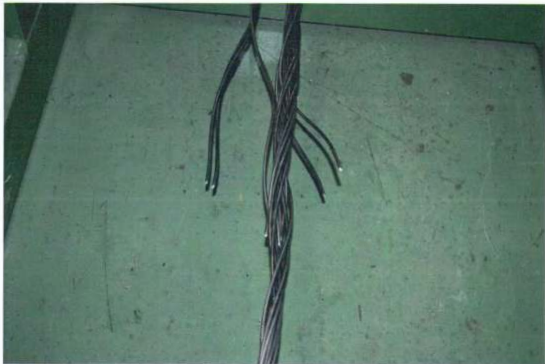
Photo 4 Fractured wires after the tensile breaking test
