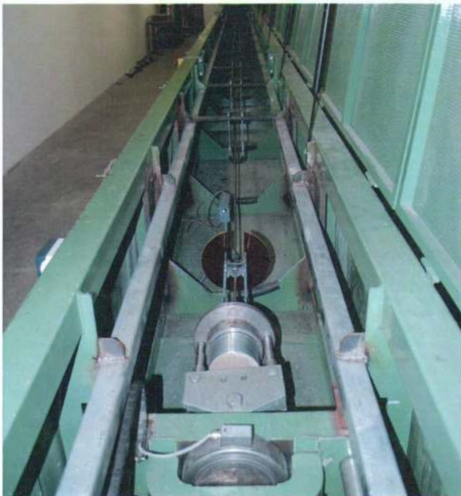
Photo 2 Stress-Strain test arrangement
