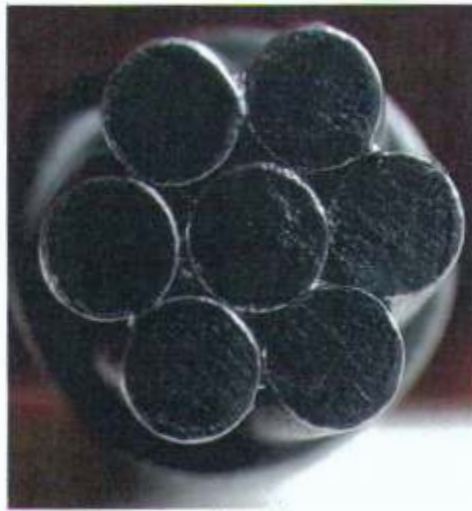
Photo 1 Cross-sectional view of the tested conductor
